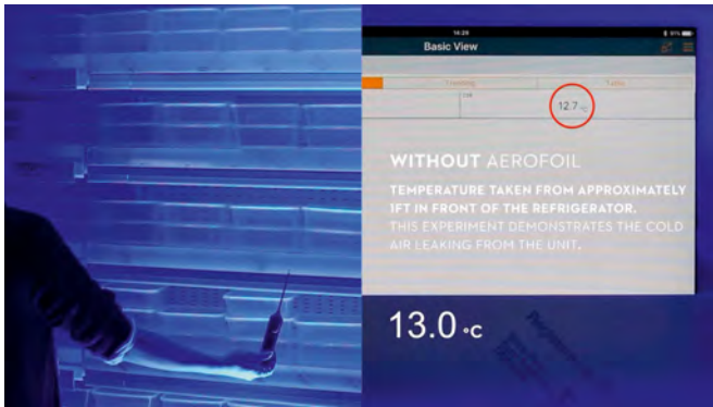
Temperature measurements taken in front of a cabinet before and after fitting Aerofoils
