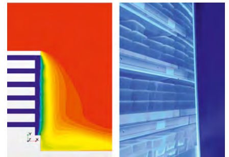
After Aerofoils are fitted to the shelves, the air-curtain is immediately straightened and more coherent in form, and very little if any cold air escapes from the cabinet.
